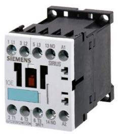
CONTACTOR, AC-3 4 KW/400 V, 1 NO, AC 24 V, 50/60 HZ, 3-POLE, SIZE S00, SCREW CONNECTION
